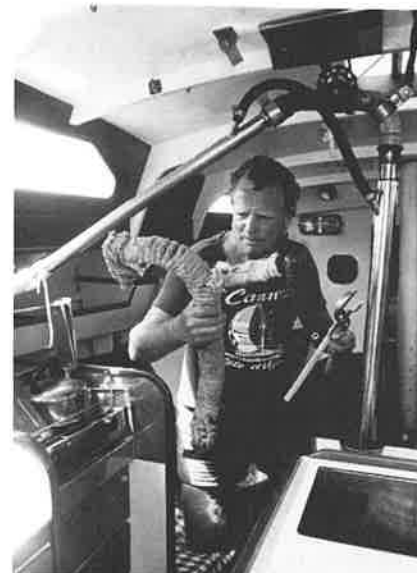
John Moody emerges triumphantly with part of KINETIC's exhaust system as he sets about removing some of the remarkable exposed interior plumbing inherited from the previous owner.
