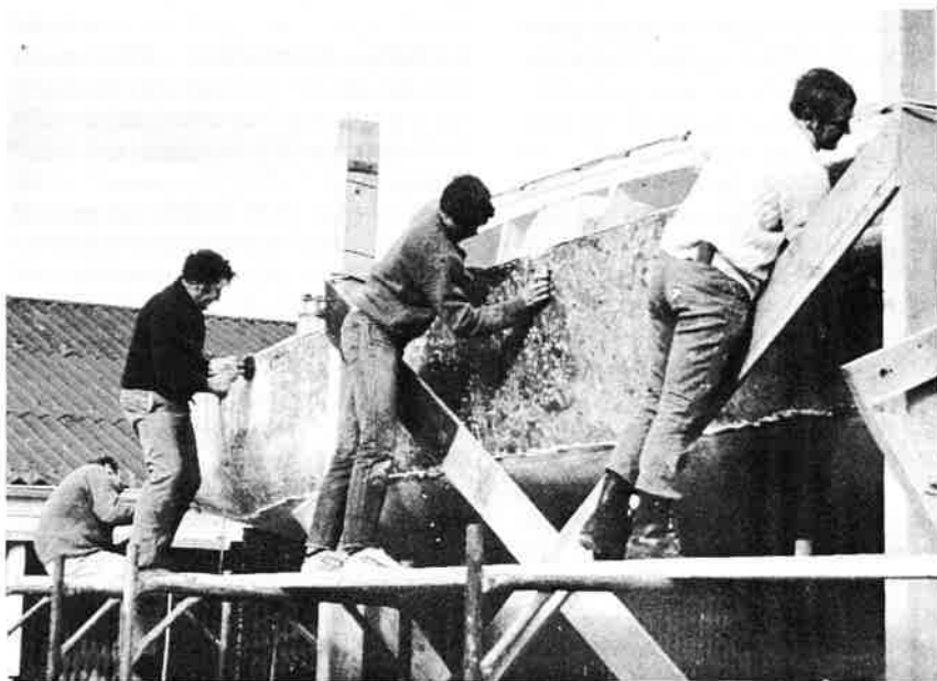
NIZAM's winter maintenance programme in full swing. The hull is being completely stripped of paint in preparation for another winning season. Hard at work are Jim Ower, skipper Graeme Hargreaves, Paul O'Shea, and Peter Lawrence.
