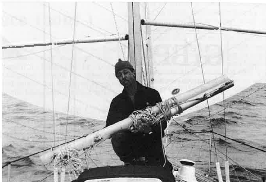
Grant Scoones holds what is left of BOBBY SHAFTO's boom, broken off East Cape on the journey to Auckland before the start of the race. They continued under poled out headsails, trys'l and motor.
